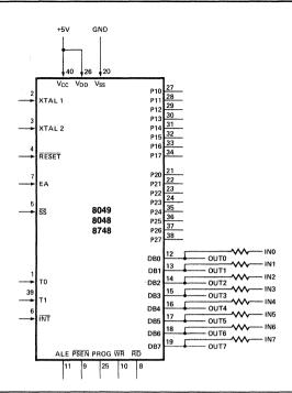
The bus is normally used as an output port. To use it as an input port the bus is put in the high impedance state using the MOVX instruction and then read using the INS instruction. The resistor value chosen is a function of the output loading and the characteristics of the input signals.
